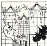
Pile stock so high that the pile blocks the water from sprinklers in case of fire.
